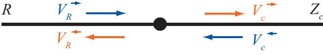
FIG. 2 (Color online) Semi-infinite transmission line of impedance Z_c terminated by a resistor R which is represented as a second semi-infinite transmission line.
